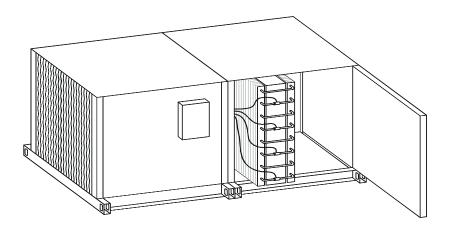
Solenoid Valve Controlled Heat Pipe System
