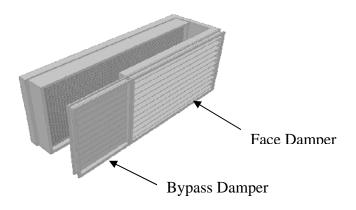
Wrap-Around Heat Pipe with Face and Bypass Dampers
