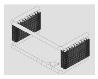
Schematic of a Manifolded Controllable Heat Pipe
