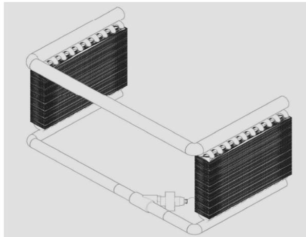
**Schematic of a Manifolded Controllable Heat Pipe**
