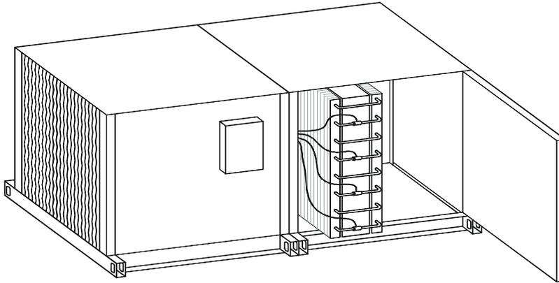
**Solenoid Valve Controlled Heat Pipe System**
