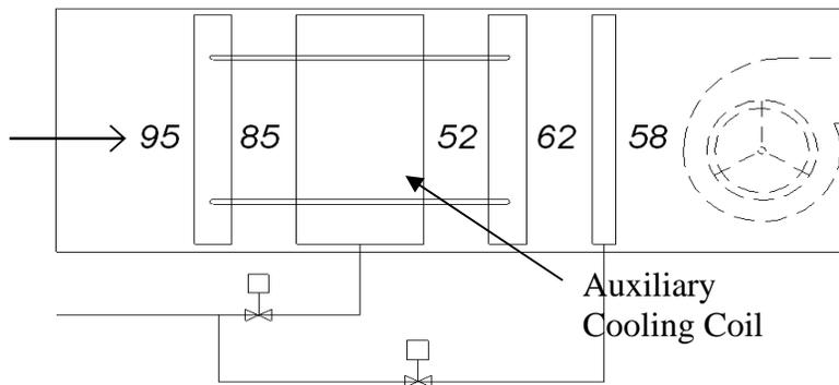
**Auxiliary Cooling Coil Schematic with Typical Air Dry Bulb Temperatures**
