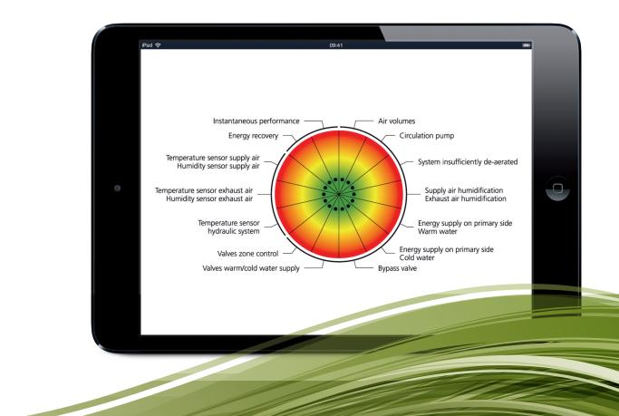
Seeing at a glance if the heat recovery system is working correctly and without error!
