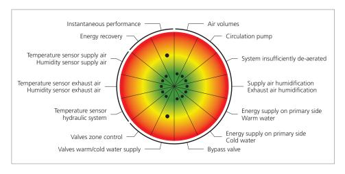
In case of a slight malfunction, the dot moves from the green to the yellow zone. The owner receives the corresponding report. In case of a serious malfunction, the dot will be located in the red zone (alarm report).
